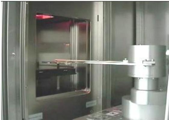
**Fig. 4: LWM9000 SEM robot unloading the reticle into the (optional) SMIF pod**
